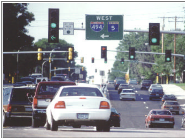
Figure 1: Example of a Permitted/Protected Phase
